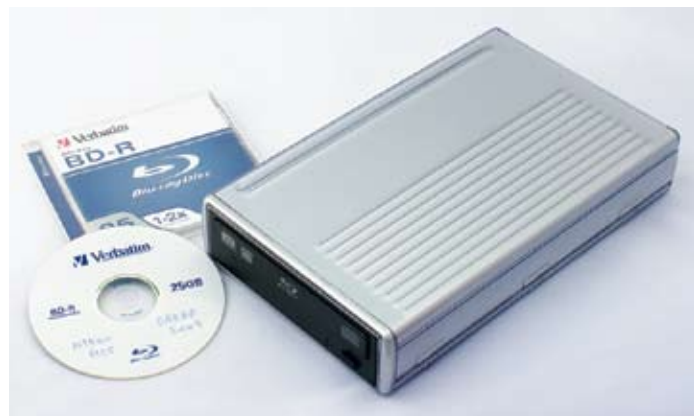
The OWC Mercury Pro Blu-ray writer can record up to 50GB on a dual-layer BD-R disc. Blank media costs anywhere from $3 to $25.
