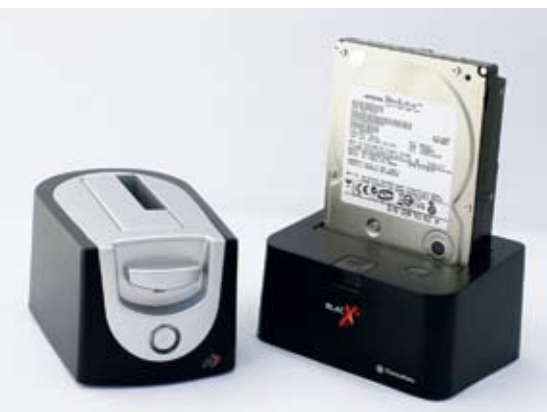
The Newertech Q (left) dock station has four different interface connections while the BlacX (right) has only a USB 2.0 and eSATA connection.
