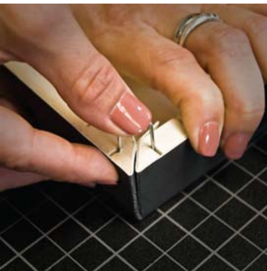
Step #8: Pull the bars up to close the frame, insert a staple into the slots and push or hammer the staple flush with the surface of the wood. Repeat on all four corners.
