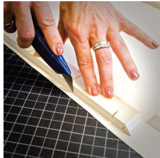
Step #4: Trim the excess print material flush with the outside edges of the stretcher bars using a sharp utility knife.
