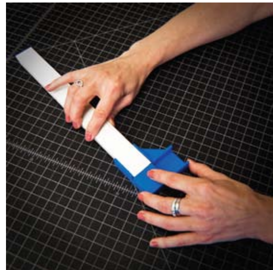
Step #1: Peel off the yellow protective strips to expose the adhesive on the bars and insert them, adhesive side up, firmly into the reusable positioning corner jigs.
