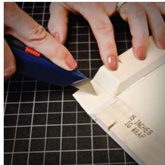
Step #6: Cut outward through the corner material at a 45-degree angle from where the bars meet.
